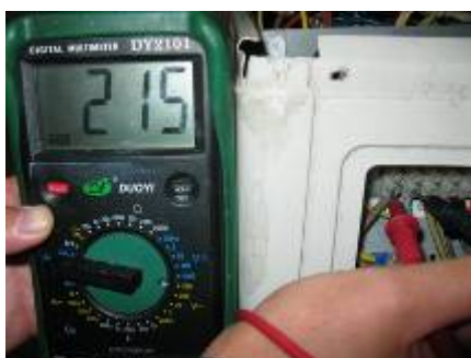
(the input voltage of the outdoor terminal)
