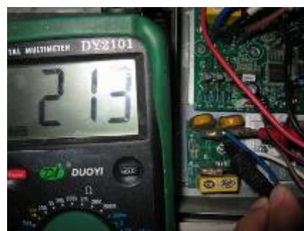
(the input voltage of the Bridge rectifier)
